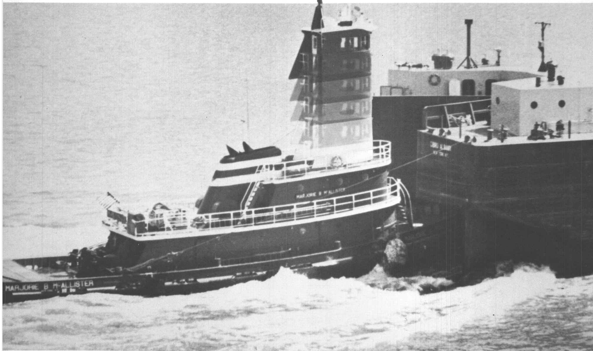
Photographic simulation of pilot house being elevated 28' height of eye to 45'.
