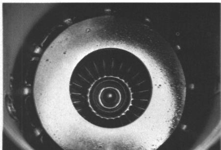
Absence of carbon or ash deposits on piston undercrowns demonstrates outstanding stability of Caprinus T and Caprinus R Oils.
