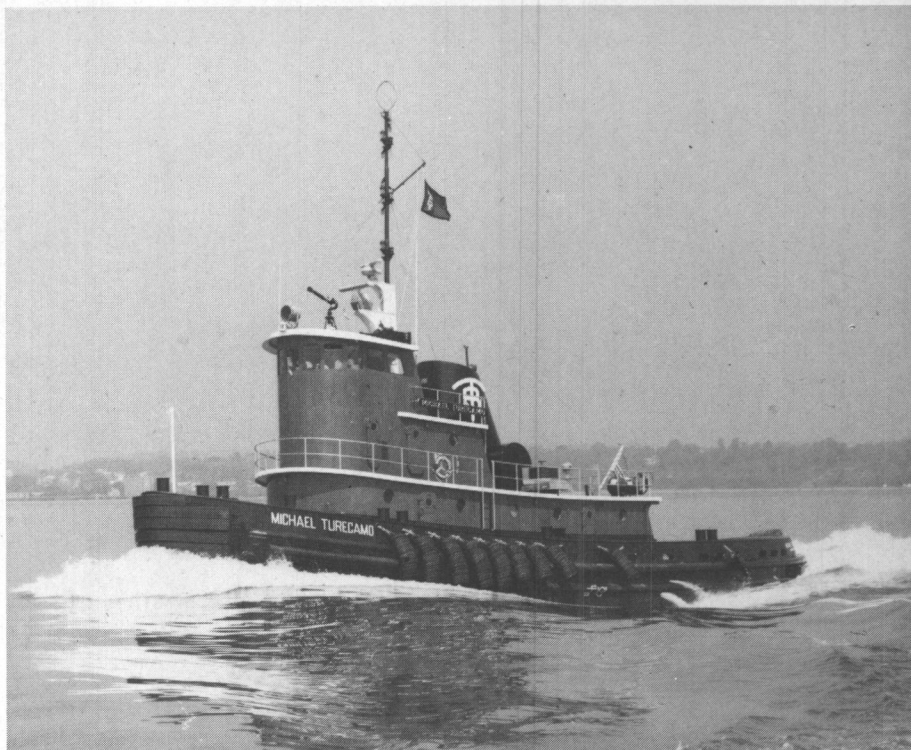
Powered by two 12-cylinder EMD 645-E2 diesels producing 2,900 shp, the 105-foot Michael Turecamo will be employed in offshore towing.
