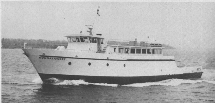
The 132-foot Munnatawket is powered by two General Motors diesels, and attained a speed of 12 knots on trials.
