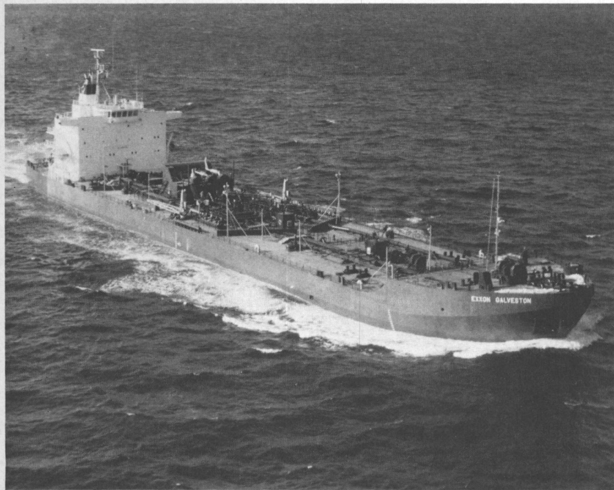
Powered by two 3,500-hp General Motors Electro-Motive diesels, the twin-screw Exxon Galveston was converted from a tug-barge unit to a tanker at Newport News Shipbuilding and Drydock Company.
