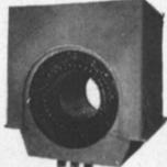
Type ATB-2 — serial #6978272. 2300/2370 volts — 60/62 cycles — 3-phase — 3600/3720 RPM — armature amps 1237/1315 — 4925/5400 KW — 1.0 PF. Westinghouse stator — from Ex "Pecos"
