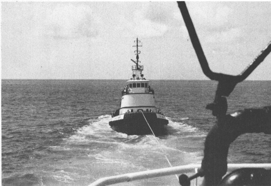
The new 6,000-hp tug Jabbar is shown utilizing the newly designed bow winches for tractor towing.
