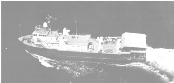
Equipped with an SCR Diesel Electric propulsion system, the geophysical research vessel Western Strait has a cruising speed of about 13 knots. The 185-foot vessel was built by Mangone Shipbuilding for Western Geophysical Company.
