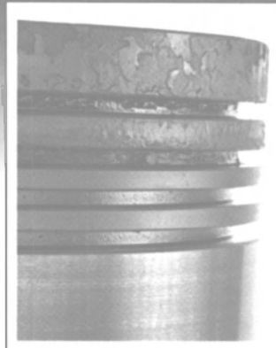
Ring groove fill normal. Number 3 and 4 lands clean.
