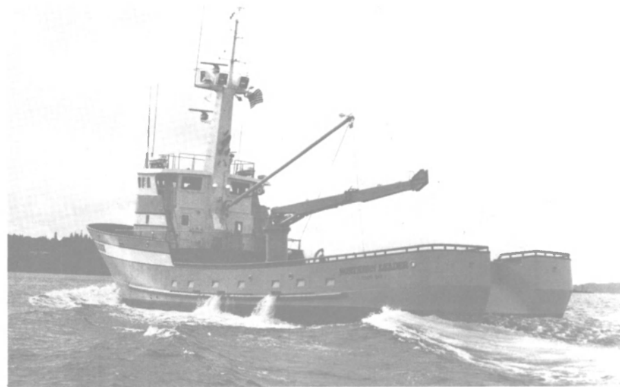
The MARCO-built 123-foot Northern Leader was recently delivered to its new owners, Tom and Colleen Peterson and Russell Ott. The vessel is equipped for all phases of crab fishing, bottom fish trawling and freezing.
