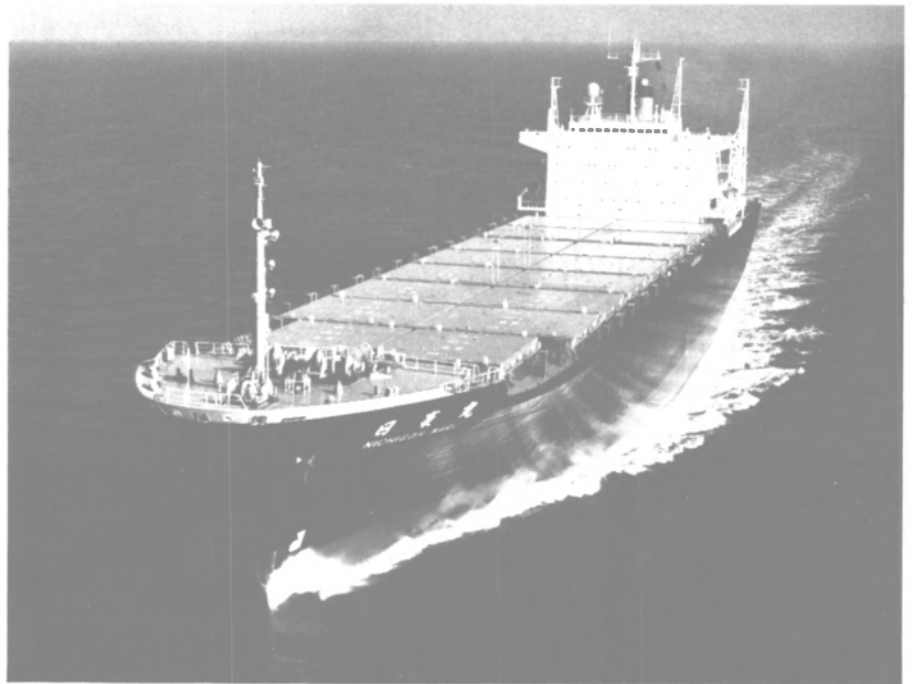
The automated containership, Nichigoh Maru, powered by a Hitachi 8L90GFC-type diesel engine, attained trial speed of up to 25.4 knots. The vessel was constructed by Hitachi Zosen at their Hiroshima Works for joint owners Yamashita-Shinnihon Steamship, Mitsui O.S.K. Lines, and Nippon Yusen.
