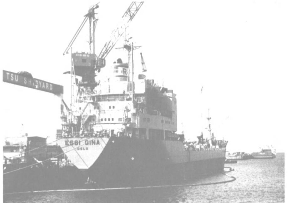
The 16.8-knot M/T Essi Gina, shown above, is equipped with a 10,200-hp, 115-rpm, Mitsui B&W 6L67GF engine.
