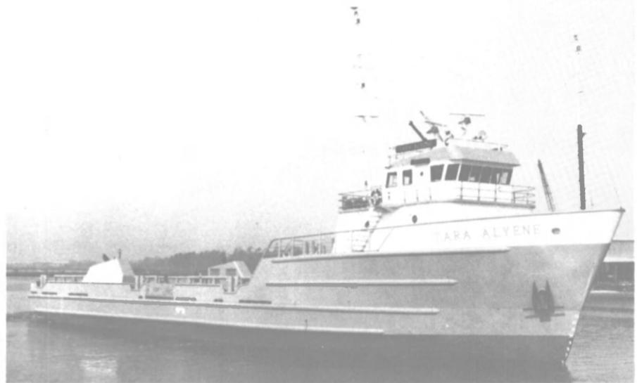
Two 900-hp GM engines and a Murray & Tregurtha bowthruster enhance the Tara Alyene's station-keeping capability.
