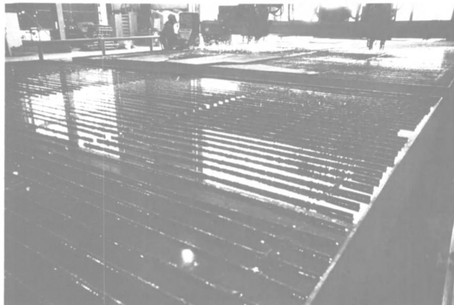
CM-100 numerically controlled plasma arc burning/cutting machine. Shown here, is the cutting of the "chocks and brackets" for the CGC Tampa, the second of four cutters under contract. It is scheduled for delivery in March 1982.
