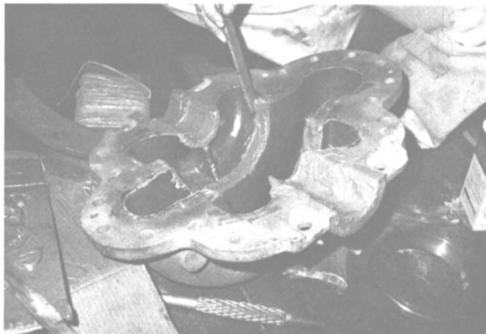
EROSION/CORROSION due to ENTRAINED SOLIDS and AIR nearly destroyed this ship's bronze pump casing. Ceramic Metal quickly rebuilt it without heat and the accompanying danger of cracking or warping the pump casing. What's more, the incredible corrosion and abrasion resistance of Ceramic Metal will increase the life expectancy of this pump by many years.
