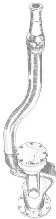
and featuring simple design, the MP provides the very high reliability required for within-tank mounting. This single nozzle tank cleaning machine weighs 178 lbs and can be fixed-in-place in any location, at any angle, and is specifically designed to allow installation on tank bottoms under the cargo.
