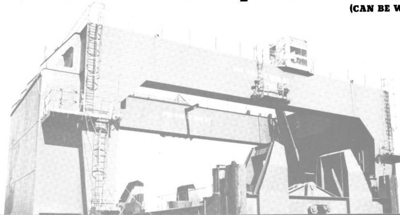
Originally Barge Handling. As used on LASH Ships. Manufactured by Alliance. Late Model built to ABS and MARAD requirements.
