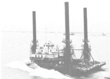
Self-propelled, jackup type well service barge Carl Fleming was launched recently at Singapore shipyard of Promet Private Limited. Positioning and emergency take-home power is provided by four GM diesels.
