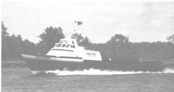
Crew/supply boat Port Arthur was completed recently by Progressive Shipbuilders & Fabricators, Inc. Built for Port Arthur, Inc., the all-aluminum vessel's four General Motors 12V71 diesels give her a top speed of 31 mph.
