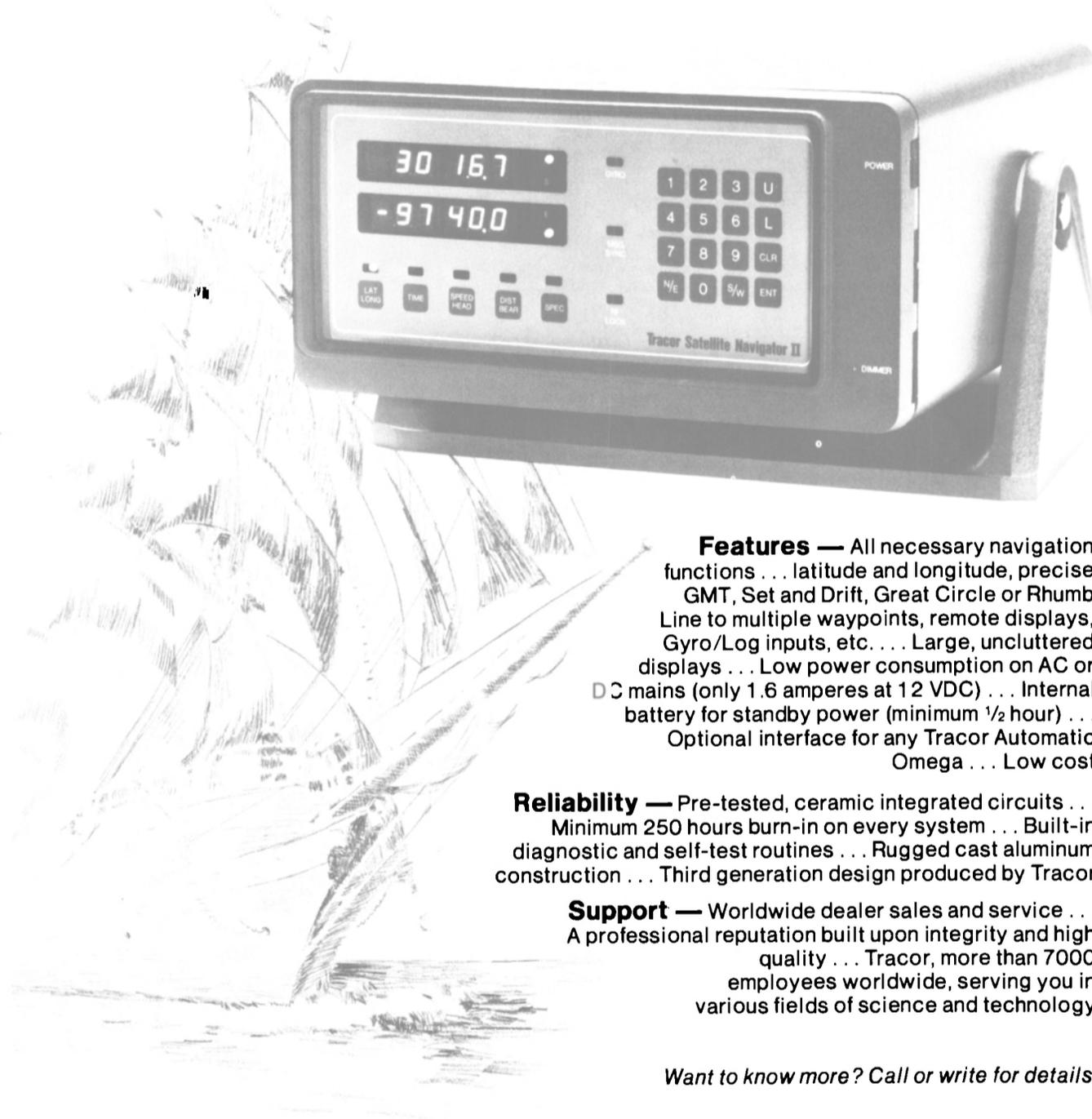
**Features** — All necessary navigation functions . . . latitude and longitude, precise GMT, Set and Drift, Great Circle or Rhumb Line to multiple waypoints, remote displays, Gyro/Log inputs, etc. . . . Large, uncluttered displays . . . Low power consumption on AC or DC mains (only 1.6 amperes at 12 VDC) . . . Internal battery for standby power (minimum 1/2 hour) . . . Optional interface for any Tracor Automatic Omega . . . Low cost
