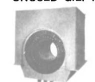
Type ATB-2 — serial #6978272. 2300/2370 volts — 60/62 cycles — 3-phase — 3600/3720 RPM — armature amps 1237/1315 — 4925/5400 KW — 1.0 PF. Westinghouse stator — from Ex "Pecos"
