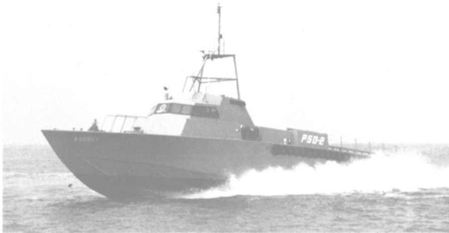
Crew/supply vessel Audrey was completed recently by Gulf Craft, Inc. for PSO Marine Transport, Inc., of Houston. Vessel's four MTU diesels drive her at top speed (unloaded) of 40 mph. Naval architect Peter Sachse calls her world's fastest planing crew/supply boat.
