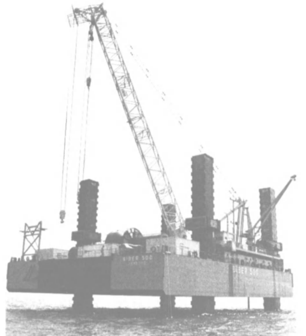
Floating crane platform Biber 500, built by Orenstein & Koppel, Lubeck, West Germany for a Hamburg owner, was designed by RSV Gusto Engineering, the Netherlands.
