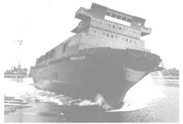
Launch of the M/V Ambassador, a 9,000-dwt roll-on/roll-off trawler ship at the Jos. L. Meyer Shipyard in Papenburg, West Germany.
