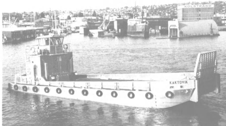
Aluminum self-propelled lighter *Kaktovik* was launched recently by MARCO Seattle. Built for Crowley Maritime, vessel is powered by three Detroit Diesel engines.
