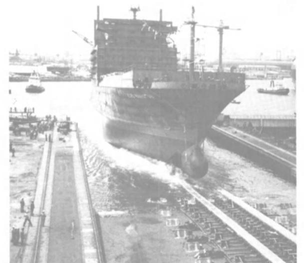
**LAUNCH IN FRANCE** — Hull No. 308, the **Ro-Ro Manhattan**, was launched recently at the French shipyard Chantiers de France-Dunkerque. The 12,640-dwt ship has a length of 170 meters and beam of 25 meters (558 by 82 feet). She is designed to carry containers, trailers, platforms, motor cars, and heavy lifts loaded as roll-on/roll-off cargoes. She will carry 684 TEUs. The ship was ordered by a subsidiary of the shipbuilder, Societe Dunkerquoise d'Armement.
