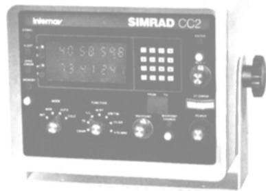
Simrad's CC-2 Navigation Computer gives complete position, steering and piloting information in an easy-to-use system. It is still the only separately packaged Loran C navigation computer, and can accept input data from any Simrad Loran C receiver.
