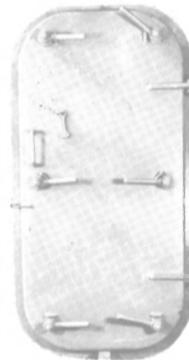
6-Dog right and left hand hinged doors with frames. Constructed of 1/4" steel plate and meet Coast Guard regulations for above deck as well as below deck use. All dogs are bronze bushed.
