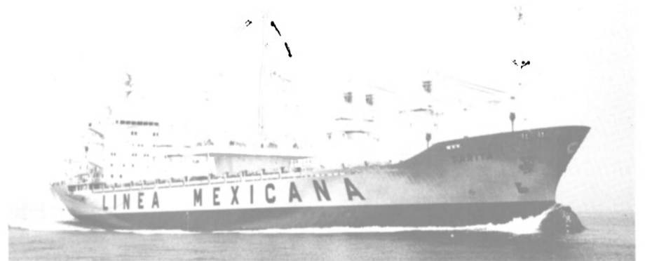
Hitachi Zosen's Hiroshima yard recently delivered the cargoliner Sarita to Callisto Shipping Ltd. Vessel is powered by fuel-saving Hitachi/B&W 8L67GFC diesel.
