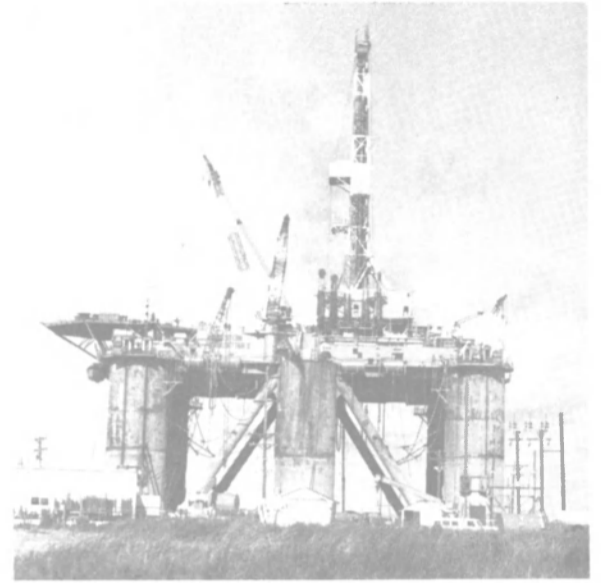
Drill rig Western Pacesetter II has been refitted by Cameron Offshore Service for operation in water depths of 900-1,000 ft. in North Sea off coast of Ireland.
