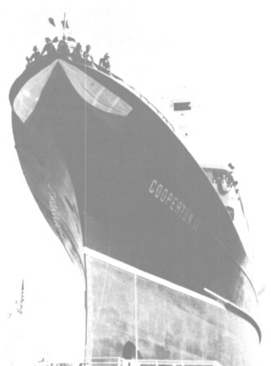
Superseiner Coopeatun II was launched recently at San Diego yard of Campbell Industries. Propulsion power is provided by General Motors EMD 3,600-bhp engine; auxiliary power comes from four Caterpillar diesels.
