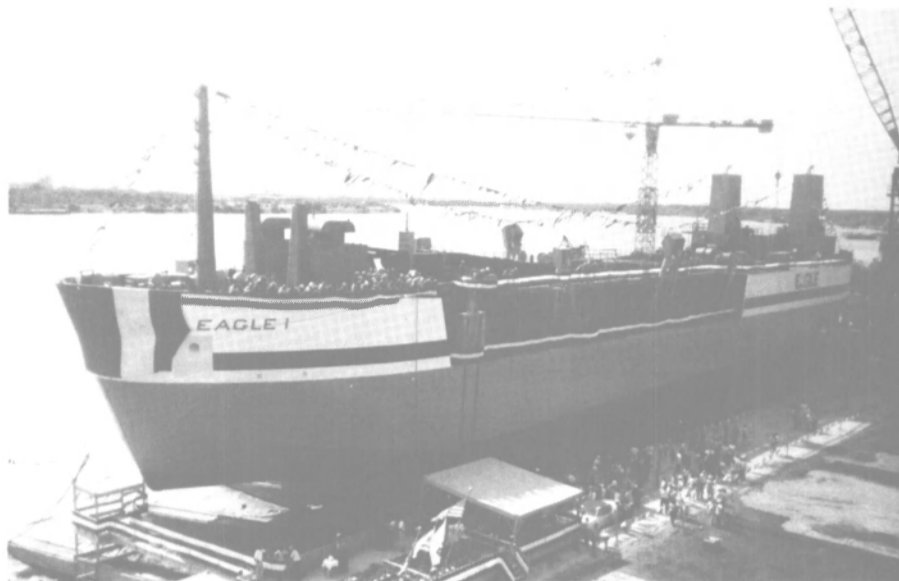
Seagoing hopper dredge Eagle I on the ways at Avondale Shipyards just prior to recent launching. Unique vessel—only five others of this type exist in the world—will be powered by two Alco diesel engines with total output of 7,500 bhp.
