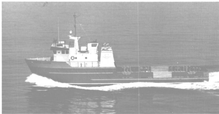
Utility vessel Wanda Louise, built by Hudson Shipbuilders for Gerald P. Hebert Enterprises, is powered by twin General Motors 16V92 NA diesel engines.
