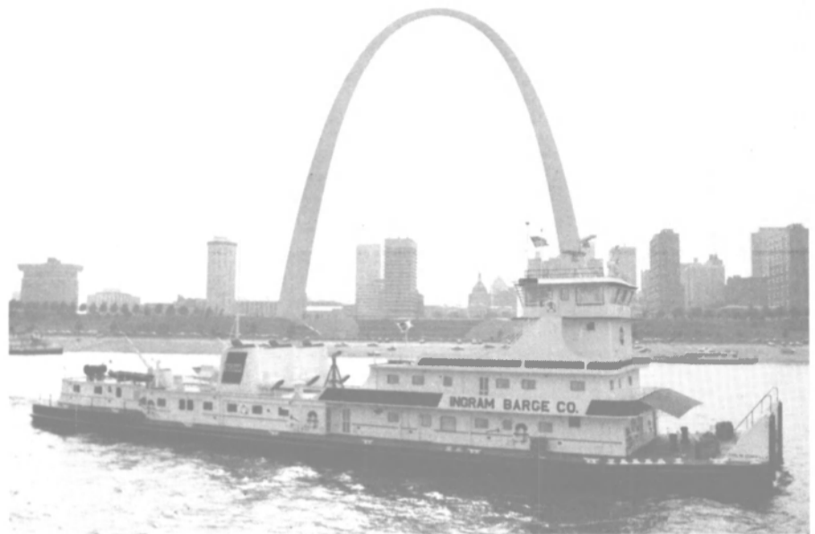
St. Louis Arch serves as background for recently christened Ingram towboat John M. Donnelly . Triple 3,000-bhp General Motors EMD diesels power the vessel.
