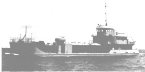
Cementing vessel Halliburton 224 was delivered recently by Rockport Yacht & Supply Company to Halliburton Services. The 130-foot vessel is powered by two Caterpillar 415-bhp diesels.
