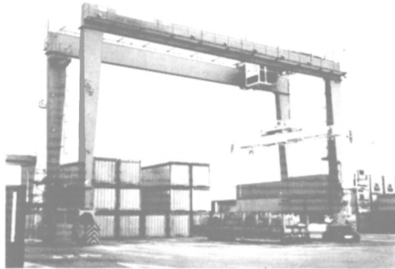
First Paceco Transtainer crane manufactured in United Kingdom by N.E.I. Clarke Chapman Cranes Ltd. is now in operation at Felixstowe Port Terminal.
