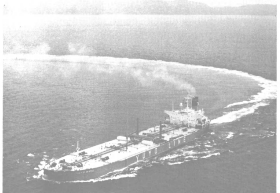
Tanker Yuhu Maru , completed recently by the Ariake yard of Hitachi Zosen, is powered by a 20,400-bhp Hitachi/Sulzer 6RLA 90 diesel that gave a trial speed of 16.6 knots.
