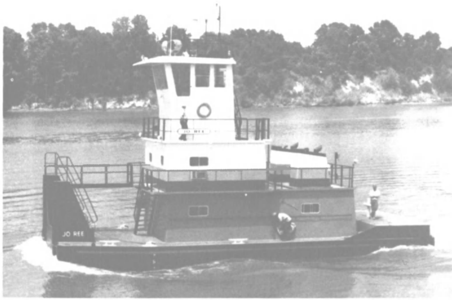
Pushboat Jo Ree , delivered recently by Dravo SteelShip to Weber Marine of Burnside, La., is powered by twin GM Detroit Diesel Allison engines with total 910 bhp.
