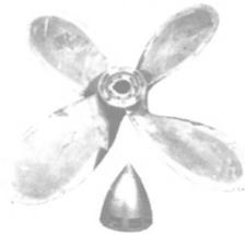
Starboard—7" diameter—pitch constant 4.699. Bore tapers from 6½" to 4¾". 14½" taper equal to 1" foot on diameter. U.S. Navy reconditioned. Average weight 1760 lbs.
