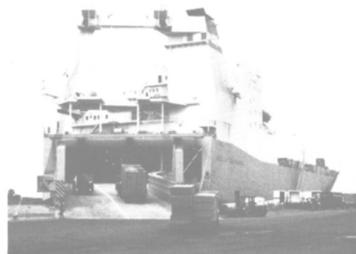
Massive quartering ramp at stern of RO/RO Hoegh Banniere was provided by Navire Cargo Gear, Gothenburg.
