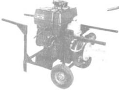
ENGINE: Mfg. by V.M.—air-cooled model HR192A—13.5 HP—3000 RPM—rope start (crank optional). PUMP: Hale—cast iron—3"—N.P.T.—hand priming—weight 410 lbs. Carrier mounted with 2 pneumatic tires for easy handling or 2-man hand carry. Ideal for oil barge, tankers, dockside, etc use.
