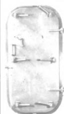
6-Dog right and left hand hinged doors with frames. Constructed of 1/4" steel plate and meet Coast Guard regulations for above deck as well as below deck use. All dogs are bronze bushed.
