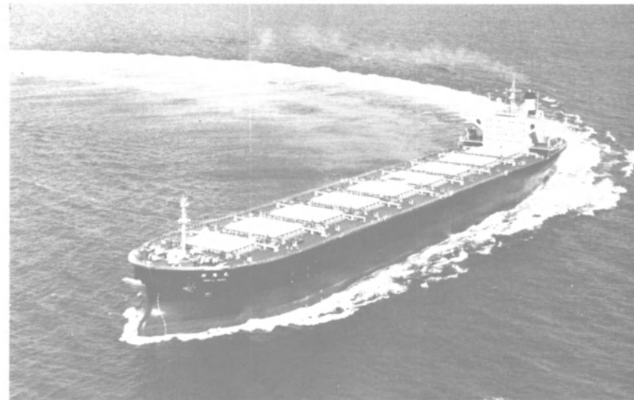
The bulk carrier Horyu Maru, powered by a 20,500-bhp Hitachi/B&W diesel, was completed recently at the Ariake Works of Hitachi Zosen.
