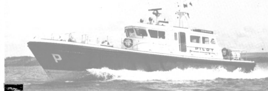
Pilot boarding launch Sullom Spindrift is an example of Rigships Limited's glass-reinforced plastic vessels that Cheverton Workboats of Cowes, Isle of Wight, will construct under license. This North Cape 65 model is powered by twin Caterpillar 3412TA diesel engines.
