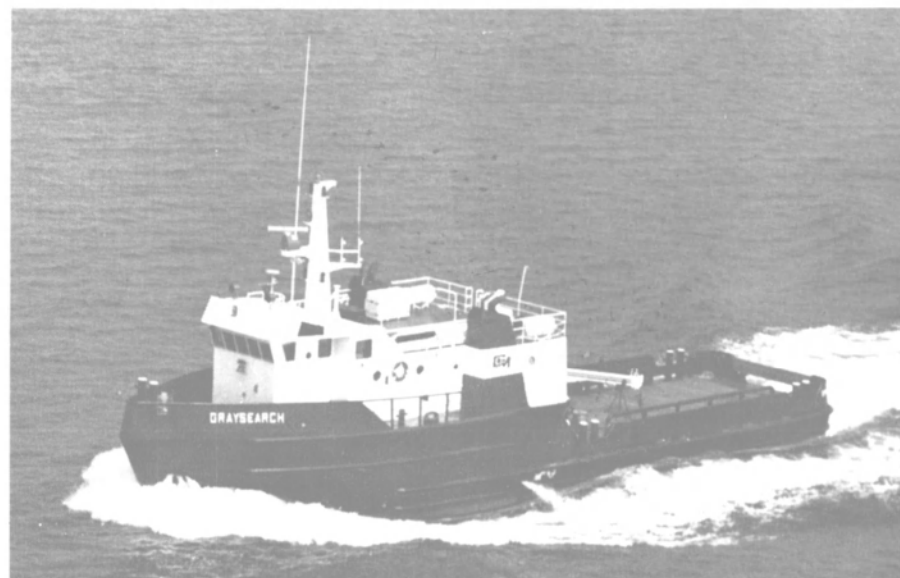
Utility vessel Graysearch was delivered recently by HUDSHIP to Gray MacKenzie Company of Bahrain. The 112-ft. boat is powered by twin Detroit Diesel 16V92 NA engines.
