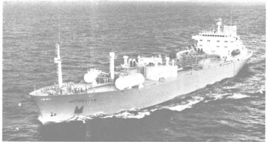
Versatile LPG/NH<sub>3</sub>/VCM tanker Hektor, completed recently by Moss Verft for A/S Nordsjogas, Stavanger, Norway, is powered by 14,400-bhp Horton/Sulzer diesel.
