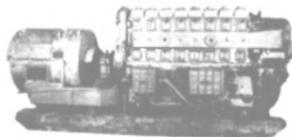
120/240 VDC—1250 amps—shunt wound. ENGINE: GM 8-268A — 8 cyl — 6 1/2 X7 — 1200 RPM — good condition.
