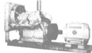
160 CFM @ 125 lbs — two stage 870 RPM — 8X8¼X8¾ — air cooled — with intercooler. Direct — connected air compressor #2261021. **MOTOR:** 50 HP 440/3/60 — mfg by U.S. Motor. **AIR COMPRESSOR:** Mfg by Air Pumps Ltd. Excellent condition — formerly used on AT&T Vessel "Long Lines" and removed only because they needed a larger unit. Complete with inter- and after-cooler. Very good condition.
