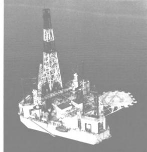
A jackup offshore drilling rig, the lle du Levant (shown above), was completed recently at the Ariake Works of Hitachi Zosen in Japan. The cantilever type rig will be operated by Foramer S.A. of France. Following delivery, the rig was towed to Abu Dhabi, where it was scheduled to begin drilling in late January.
