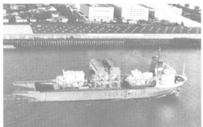
Outbound from Port of New Orleans, heavy-lift ship Dock Express 12 has deck load of three offshore production modules bound for Bahrain.
