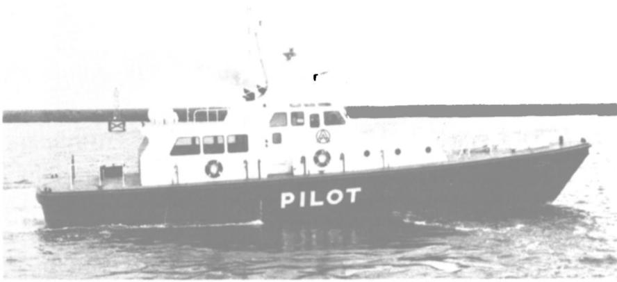
Pilot boat Elalat 9, delivered recently by Halter Marine to Marine and Transportation Services (Saudi), Ltd., is powered by twin Detroit Diesel engines developing total of 1,700 bhp for speed of 20 mph.
