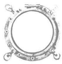
Recently carefully hand removed from ocean vessels. Suitable for re-use on shipyard conversions or for marine ornamental use. Heavy marine standard glass . . . clear or can be furnished frosted for use in special locations.
