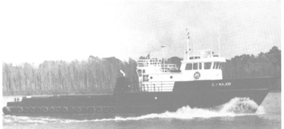
Rugged utility vessel C/Major was completed recently by Swiftships for CO-MAR Offshore Corporation. The 115-foot craft is powered by twin Detroit Diesel 16V149N engines with total output of 1,350 bhp.
