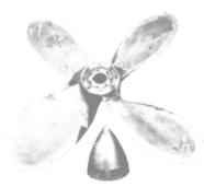
7' Diameter—pitch constant 4.699. Bore tapers from 6 1/8" to 4 53/64". 1412" Taper equal to 1"/foot on diameter. U.S. Navy reconditioned. Average weight 1760 lbs.
