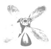
Starboard -7' diameter - pitch constant 4.699: Bore tapers from  $6\frac{1}{4}$ " to  $4\frac{5}{4}$ 4".  $14\frac{1}{2}$ " taper equal to 1"/foot on diameter. U.S. Navy reconditioned. Average weight 1760 lbs.
