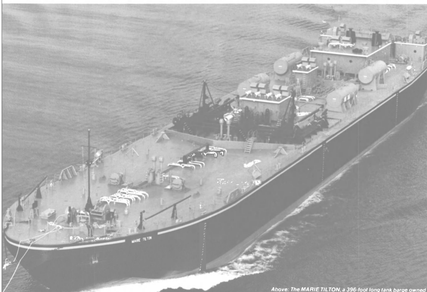
Above: The MARIE TILTON, a 396-foot long tank barge owned by Turecamo Tankers, Inc. Designed with a 103,500-barrel capacity, the TILTON features a flexible cargo handling system which allows it to carry multiple cargoes and has an off-loading capacity of 18,000 barrels per hour.
