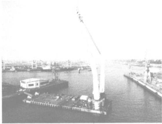
The 900-ton, heavy-duty floating derrick Tog Mor (shown above) was delivered recently by Blohm + Voss AG, Hamburg. Built for Howard Doris Ltd. of Edinburgh, the derrick's hull is 101.4 meters long and 27.4 meters wide (about 332.7 by 89.9 feet). It has been towed to Loch Kishorn yard in Scotland.
