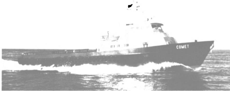
Gulf Craft Inc. custom built the Comet to Shippen's specifications. The aluminum-hulled quad-screw is capable of 23 knots and is the first crewboat to be powered by four Cummins KTA-1150-Ms.
