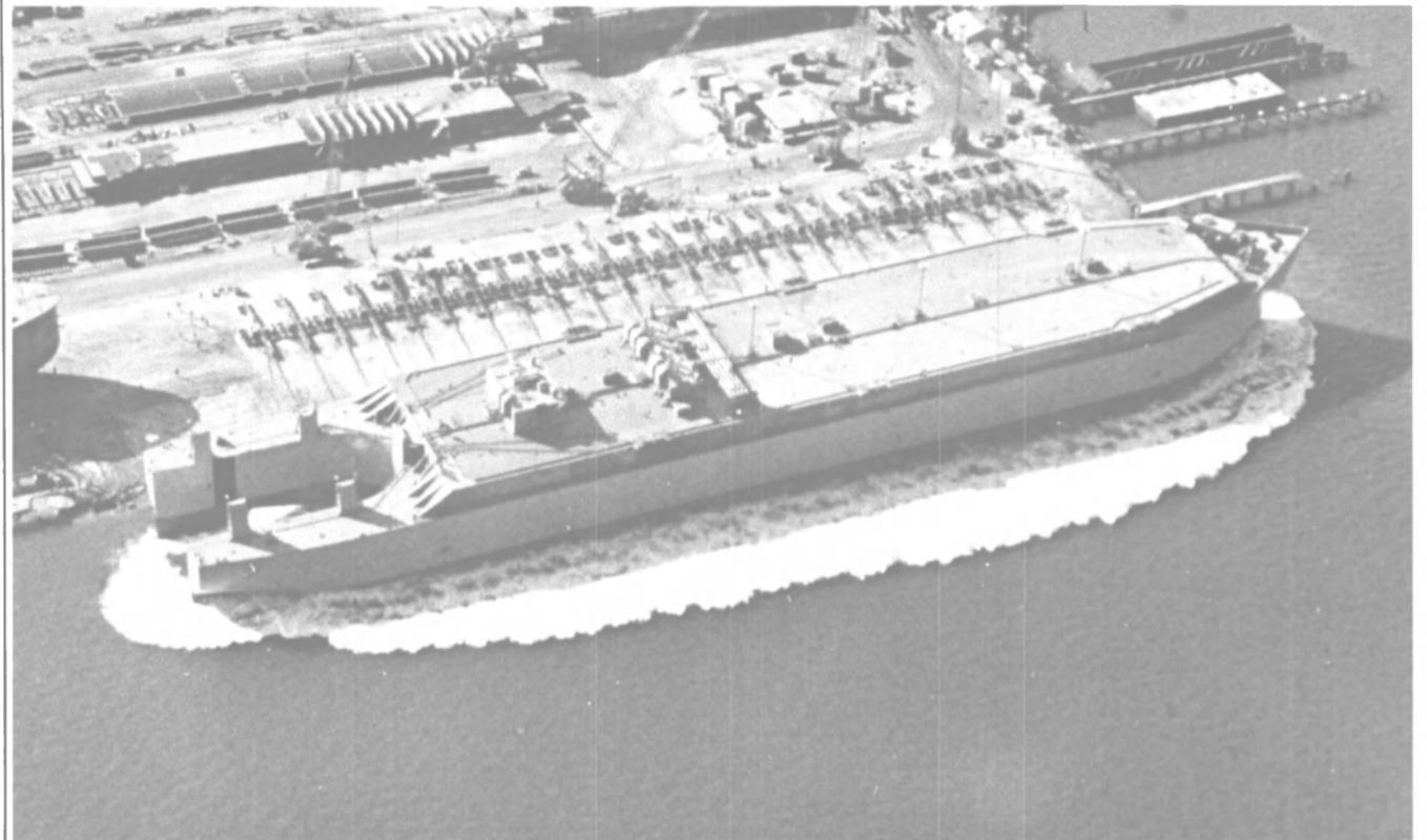
**BELCHER 102-BIG AND VERSATILE.** The biggest barge ever built in this country for the transportation of oil and probably the largest ever constructed anywhere for the movement of petroleum products. Double skinned with dimensions of 640 feet long by 105 feet wide and 48 feet deep, she has a capacity of 55,000 DWT or 412,000 barrels.
