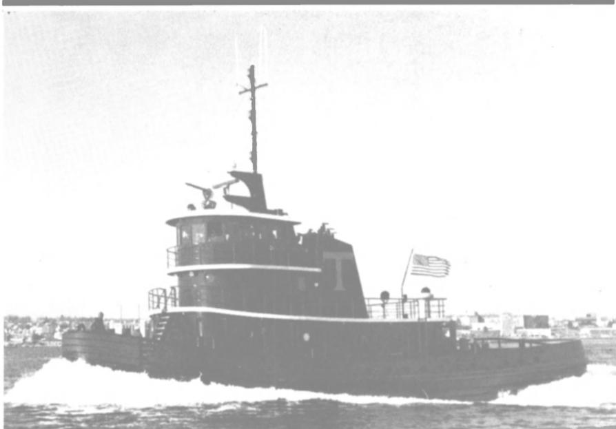
The Paul A. Wronowski was designed for docking nuclear subs and other large vessels at the U.S. Naval Base in Groton, Conn. The 90-foot tug was built by Thames Shipyard in New London, and is the first boat outfitted with 16-cylinder Cummins KTA-3067 engines.
