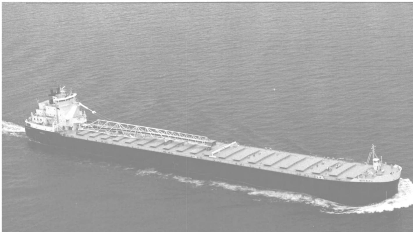
Above: The M/V BUFFALO, a 635-foot long self-unloader built for American Steamship Company, Buffalo, New York. Designed with an unloading rate of 3,500 short tons of coal per hour or 6,600 long tons of ore per hour, the M/V BUFFALO has a cargo deadweight of 23,110 long tons.
