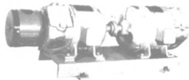
2 1/2 KW—115 volts single phase A.C. output. GENERATOR: Type GNA—class 1G— Frame 28A—Form A—1800 RPM—5 KVA—2.5 KW 115 volts AC— 60 cycle —50% PF—43.4 amps. MOTOR: Louis Allis—Type GNA—Class E—Frame 25A—Form A—1800 RPM—115 volts DC—32 amps—shunt wound (with attached Ward-Leonard frequency regulator). Some control panels available.
