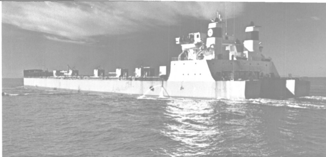
The M/V SEABULK MAGNACHEM, and her sister ship the M/V SEABULK CHALLENGER (above) are 39,000 ton integrated tug/barge combinations, transporting bulk liquids between U.S. Gulf and Atlantic Coast ports.
