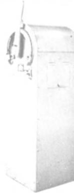
For 12-567A engine and Falk reduction gear. As used for USN LST vessels. Bridge and engine room control.
