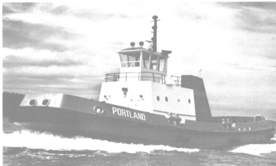
Shaver Transportation Company has recently taken delivery of a new ship handling tug, the Portland, for service in the Port of Portland. The Portland is propelled by two Maritime Industries model 1650 H 360° steerable Z-drives, each rated at 1,700 bhp. The Maritime propulsion units are believed to be the largest currently installed in North America for tug application.
