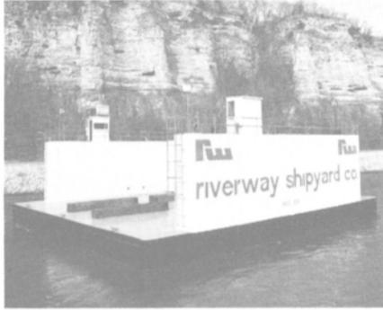
Riverway Shipyard Company of Grafton, Ill., recently completed its second in-house drydock (shown above) for the repair division of the shipyard. This drydock is the fourth built by the shipyard in the past two and one-half years and was built in a record 86 calendar days. It went into immediate service drydocking two harbor boats.
