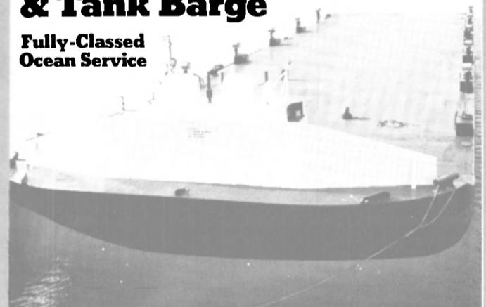
**ZPC-402** 230' x 60' x 15' Comb. Deck Cargo & Grade 'D' Tank Barge
