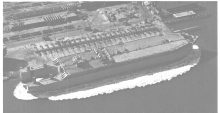
**BELCHER 102-BIG AND VERSATILE.** The biggest barge ever built in this country for the transportation of oil and probably the largest ever constructed anywhere for the movement of petroleum products. Double skinned with dimensions of 640 feet long by 105 feet wide and 48 feet deep, she has a capacity of 55,000 DWT or 412,000 barrels.
