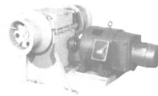
2500 LBS @ 125 FPM on one gypsy head or 1250 lbs @ 125 FPM simultaneously on each gypsy. MOTOR: 15 HP—230 volts DC—55 amps—GE. AVAILABLE: 1 Set mfg by Lakeshore with Reliance motor—1 set mfg by Ideal with GE motor. Complete with controls and disc brake.
