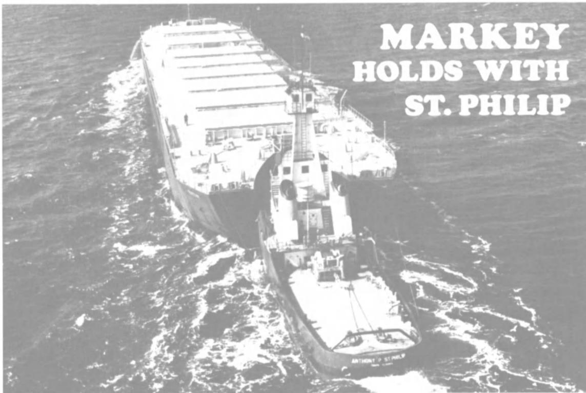
Tug ANTHONY P. ST. PHILIP (and sister ALICE ST. PHILIP) are equipped with Markey Towing Winch, Capstans and Anchor windlass. These twin screw 5600 horsepower St. Philip
