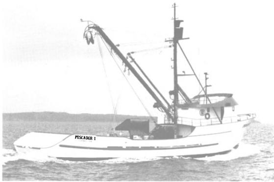
Pescador I by MARCO is powered by a Caterpillar D398TA diesel driving a Coolidge bronze propeller.
