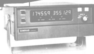
**TL-838 Loran C Receiver** simultaneously displays two lines of position from automatically acquired and tracked masters and all available Loran C secondaries. TL-838 has four tunable and two preset notch filters for outstanding performance, worldwide. It incorporates a three point memory, and *very fast acquisition and setting.*
