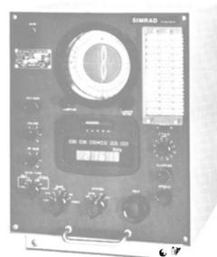
**Two IMCO approved automatic direction finders,** the TD-A202B and the TD-C328HATS (shown), are now offered by Simrad. The TD-A202B has frequency ranges of 200-580 KHz beacon band and 1.5-2.8 MHz marine band. The TD-C328HATS has a range of 200 KHz to 13.5 MHz. Both are highly sensitive superheterodyne receivers. *They lock in fast.*
