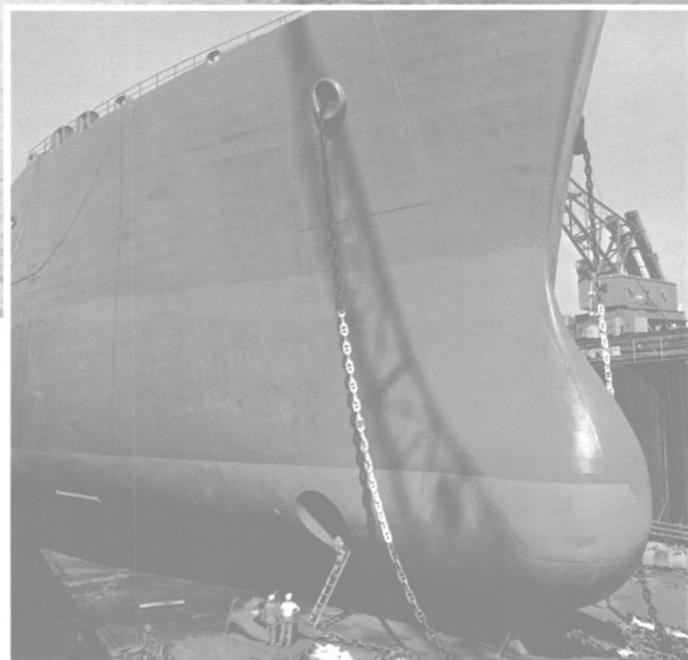
*The boot-topping and freeboard areas of this tanker have been painted with a coating system that includes a two-component aliphatic urethane topcoat based on Desmodur N and Desmophen urethane resins from Mobay.*
