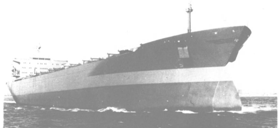
The M/S Baumare, recently delivered by B&W Shipyard to Baumare Inc., is powered by a five-cylinder long stroke B&W type L80GFCA engine.
