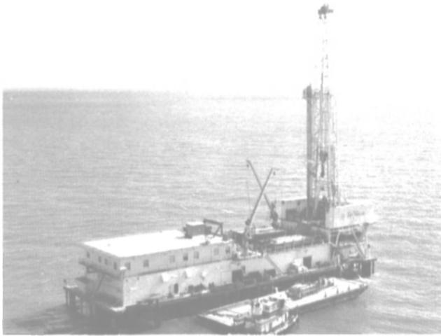
At work for the Louisiana based Circle Bar Drilling Company is the posted drill barge Pat Taylor. It is rated to work drilling depths of up to 30,000 feet.
