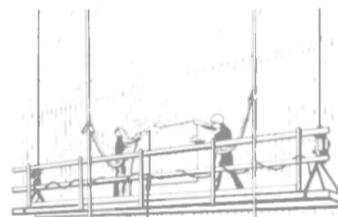
Platform for interior and exterior wall work
