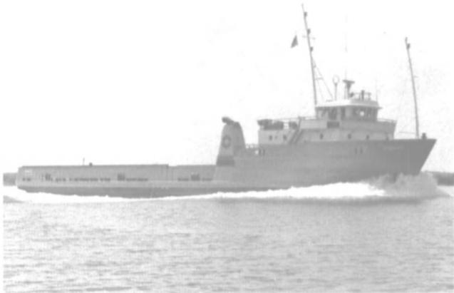
At work offshore for Petrobras is the Rincao, 185' by 38' with a 16' depth. This tug/supply vessel is one of five built for Brazil.
