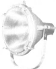
HEAVY DUTY CAST ALUMINUM marine floodlights—series 48116—ADE 16. U.L. Marine listing 595—also USCG accepted. Mogul base—will handle 1000 watt incandescent or clear metal Halide bulb. Corrosion-resistant—hinged door.
