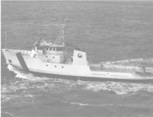
At work offshore for NASA is the UTC Freedom, 176' by 37'. Designed to recover the space shuttle's rocket booster, this vessel and her sister ship, the UTC Liberty, can also accommodate a variety of scientific and technical missions.
