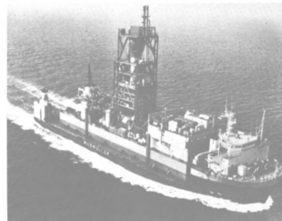
The world's first transportable polyethylene plant en route from Japan to Bahia Blanca, Argentina.
