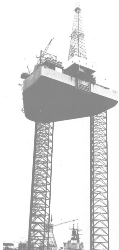
**SITTING ON TOP**—The Keyes 301, the second L-780 self-elevating offshore drilling unit to be built for Keyes Offshore Companies, Houston, Texas, by Ingalls Shipbuilding, Pascagoula, Miss., is jacked to the top of its 390-foot legs during successful testing operations prior to recent delivery. The unit is now drilling for ARCO Oil and Gas Company off the Louisiana coast. Ingalls, the third largest rig builder in the country, has 14 additional units under contract, including two more for Keyes.
