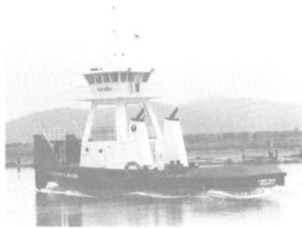
Mid-Coast Marine, Inc. of Coos Bay, Ore., announced the recent delivery of a 72-foot twin-screw towboat, Clemente Guillen (shown above), to Roca Fosforica Mexicana SA de CV of Mexico City. The vessel was designed by David J. Seymour, Ltd., naval architect of San Francisco, Calif. Home port will be Lopez Mateos, B.C.S.
