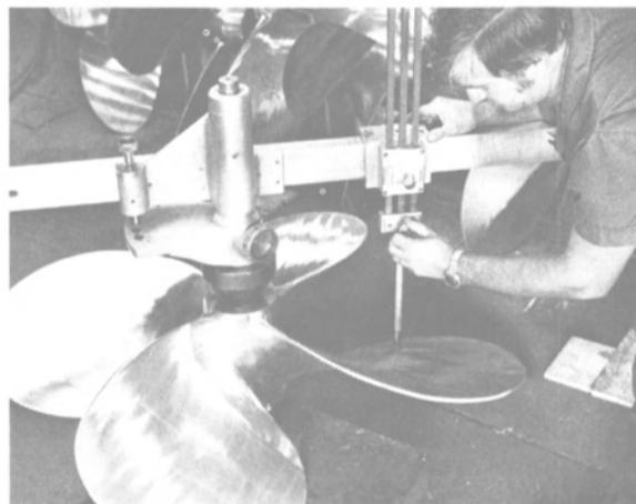
Michigan's Work-Horse™ is a tough 4-blade propeller with heavy cross-sections and heavy-duty leading edges designed to give you smoother operation than the 3-blade wheel it replaces. It is cast and available in three very strong materials: Michalloy K bronze and Ni-Bral through 30' dia., and CF 3 mod Stainless Steel in sizes through 18' dia. All offer exceptional resistance to corrosion and damage... could save costly haul-outs, repair and downtime.
