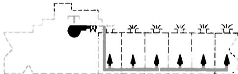
Complete systems for new-buildings or retrofitting. All components designed and manufactured in the United States, consisting of flue gas valves, scrubber, motor or turbine fan packages, gas regulating valve, non-return valve, deck water seal, and main control panel. Optional: auxiliary control panels, fan isolation valves, deck valves, etc. Complete system designed for specific vessel's requirements.
