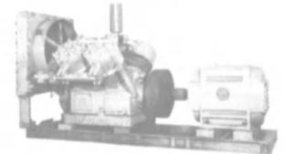
160 CFM @ 125 lbs — 2-stage 870 RPM — 8 X 8 1/4 X 8 3/4 — air cooled — with intercooler. Direct-connected air compressor #2261021. MOTOR: 50 HP 440/3/60 — mfg by U.S. Motor. AIR COMPRESSOR: Mfg by Air Pumps Ltd. Excellent condition — formerly used on AT&T Vessel "Long Lines" and removed only because they needed a larger unit. Complete with inter- and after cooler. Very good condition.
