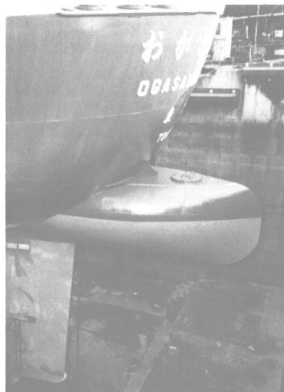
Kawasaki stern end bulb protrudes from center line of hull near full-load waterline. In test installation, this ship recorded 5 percent saving in propulsion.
