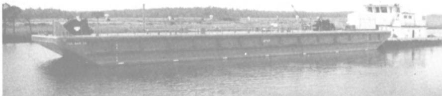
The 160-foot-long tank barge Tide Mar 34 can transport 10,500 barrels of oil and is also fitted to carry deck cargo.
