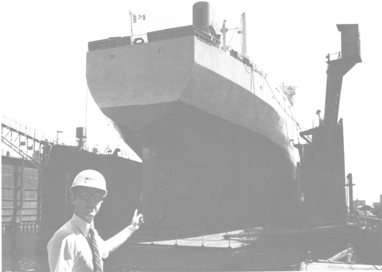
The *Irving Arctic*, squeezed into Dock No. 1 at Bethlehem's Boston Yard. Workmen repaired damage to the hull with less than 3 feet to move around in—the distance between the ship's sides and the wingwalls.
