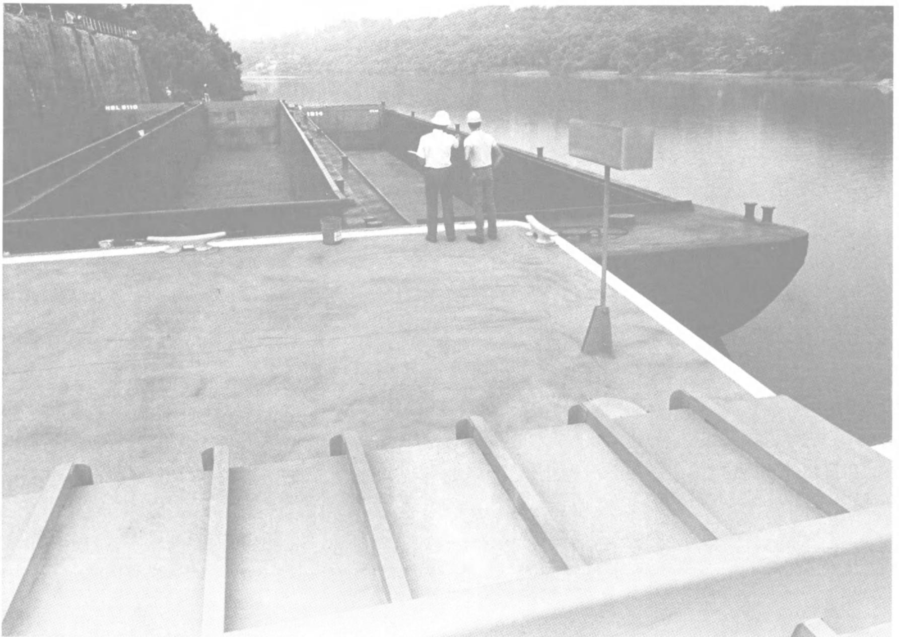
For two upriver coal customers with different operations: upper left, two 195 x 26 x 11 barges; right, a 170 x 20 x 11 barge; foreground, 195 x 35 x 12 hazardous cargo tank barge.
