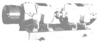
2½ KW—115 volts single phase A.C. output. GENERATOR: Type GNA—class 1G—Frame 28A—Form A—1800 RPM—5 KVA—2.5 KW 115 volts AC—60 cycle—50% PF—43.4 amps. MOTOR: Louis Allis—Type GNA—Class E—Frame 25A—Form A—1800 RPM—115 volts DC—32 amps—shunt wound (with attached Ward-Leonard frequency regulator). Some control panels available.
