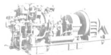
GENERATOR: Westinghouse 450KW 563KVA—450/3/60 721 amps — 80% PF — 1200 RPM — serial nos. 2 519P405 & 6 519P405. GEAR: Worthington-Moore — form 14 x 10 — gear 1200 RPM — pinion 6097 RPM — ratio 5.08:1. Serial Nos. 7801 & 7802. TURBINE: Worthington — 250 lbs steam @ 406° — form U356 — exhaust 27.5" vac. — shop order 4161 — serial Nos. 7801 & 7802.
