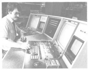
Traffic and cartographic data in the radar-surveilled area will be shown as color pictures on four display consoles in the port operational center of Gothenburg, Sweden. The VTM system, using the very latest microprocessor technology in processing data, is developed by Norcontrol of Norway.
