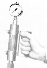
ATTACHES TO STANDARD INDICATOR VALVE INDICATES CHANGE IN CYLINDER LOAD WHILE ADJUSTING FUEL RACK GAUGE READING COMPARABLE TO AREA OF INDICATOR CARD SIMPLE TO USE REQUIRES NO MAINTENANCE ACCURATE RELIABLE
