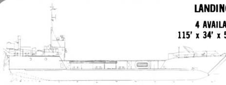
**CARGO CAPACITY: 167 TON / FULL LOAD DISP: 347 TON / CONSTRUCTION: WELDED STEEL—FLAT BOTTOM / FUEL CAPACITY: 11 TONS (3,542 Gal.)
