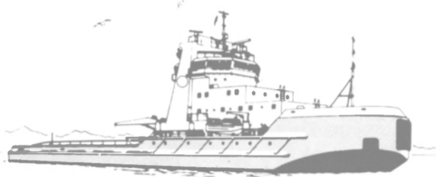
259' Arctic Supply Vessel, 1250 HP OMNITHRUSTER with Ice Field Hull Lubrication**
