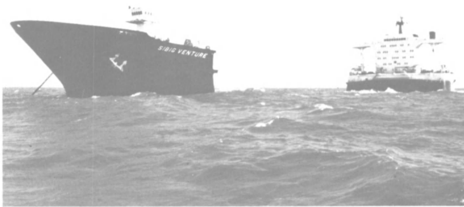
The Sibig Venture submerged to a draft of 15 meters during immersion trials in Cadiz Bay, Spain.
