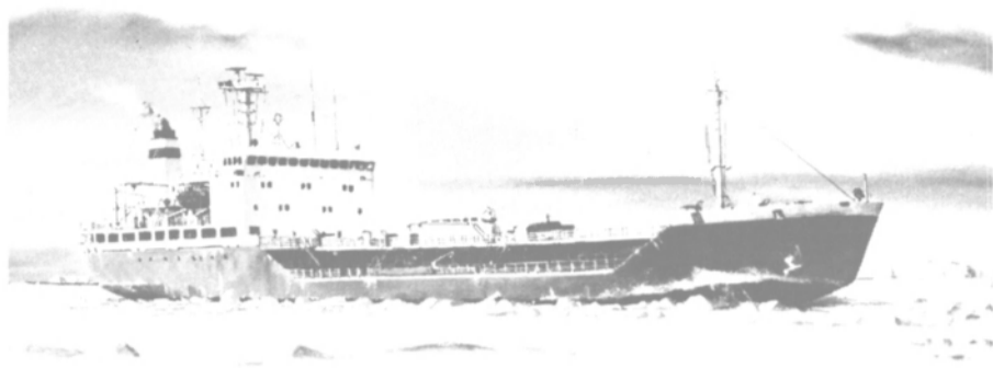
Artist's rendering of The Ventspils. The Arctic-class product carrier is powered by a slow-speed B&W diesel engine.
