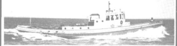
94' L.O.A.; 24' Beam; 13'-6" Depth; Welded Hull; Ice Reinforced Bow; 1000 SHP; 1200 HP 12-278A GM Engine; Built Defoe 1952; Bronze-line Shaft; Steel Propeller; Radiophone FM Modar Triton, 12 Channel; Radar; Gyro; Last docked June 1978; Cook and Sleep Facilities. Lying at Rogers City, Michigan, United States Steel. Contact
