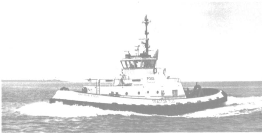
The tug Arthur Foss features a Voith-Schneider cycloidal propulsion system powered by two EMD diesel engines.
