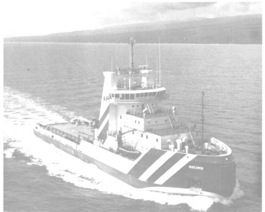
The M/V Miscaroo can operate in 4 feet of ice at 3 knots
