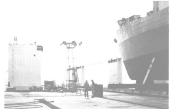
This floating drydock at Daewoo's Okpo yard employs a Hydranautics Hydraulic Systems innovative ship transfer system.
