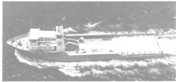
The Nicor Power built by Moss Point Marine is powered by EMD engines totaling 6,000 hp.
