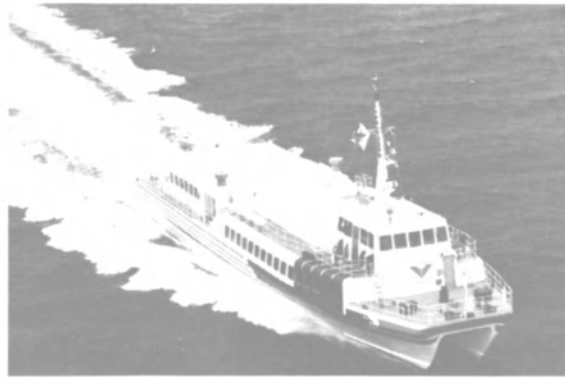
The 280 passenger catamaran ferry Marine Hawk showing its high speed capability.
