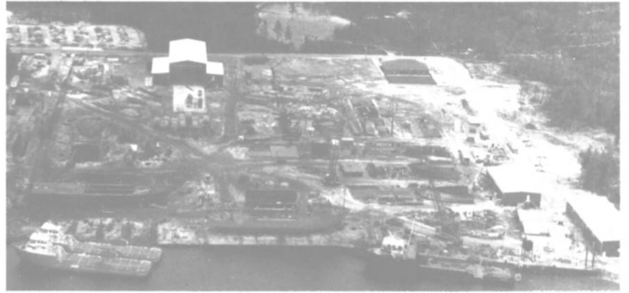
Moss Point Marine's modular construction system enables a vessel to be constructed in different sections simultaneously on their 21-acre site on the East Pascagoula River.
