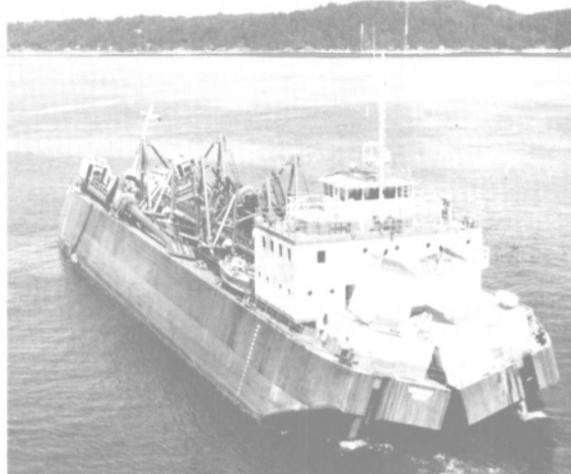
Unfolding, the split-hull self-propelled hopper barge Newport dumps its load.
