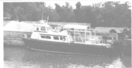
42' x 14' x 7' Aluminum Crewboat, Built 1981 by Bayou Black Shipyard, twin GM 6-71 engines, 600 HP, 10 KW Generator, 16 Passenger, excellent condition.
