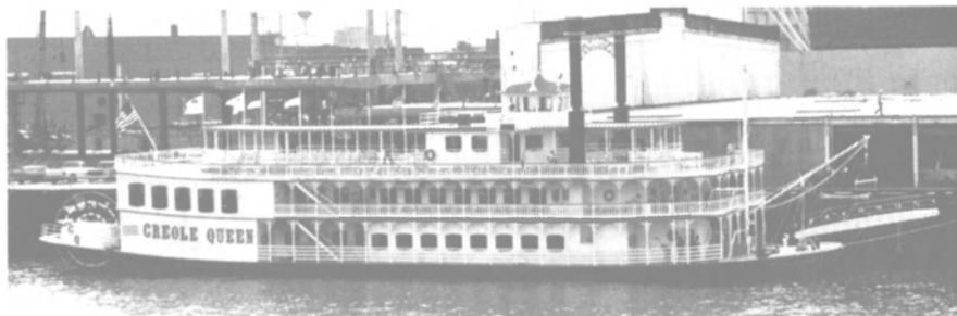
This diesel-electric powered paddlewheeler uses Caterpillar engines, GE generators and Reliance drive motors.
