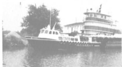
46' x 15' x 6' Aluminum Crewboat, Built 1981, Delta Bay Craft Shipyard, Twin GM 8-V-92 engines, 600 HP, 10 KW Generators, 28 Passenger, excellent condition.
