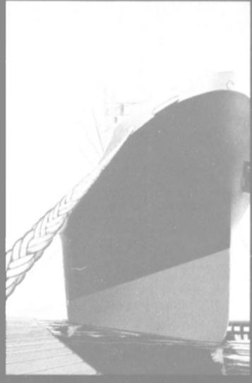
STEEL LINE is available in 3 or 8-strand construction, in diameters 1½ inches and larger. And it's manufactured in the United States from domestic materials.
