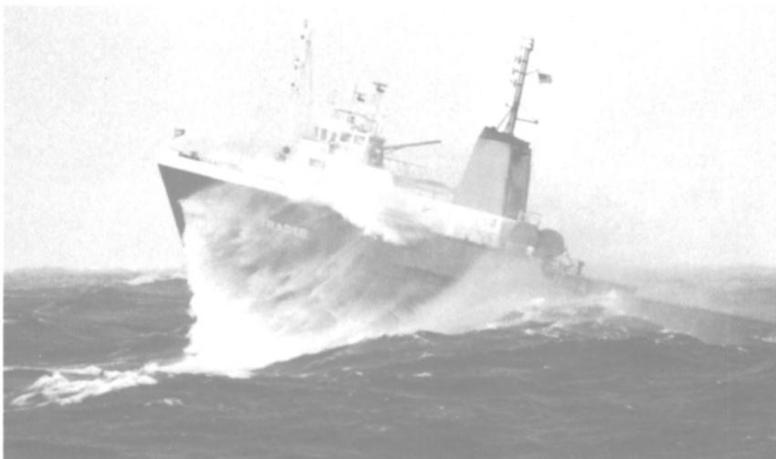
Transamerica Delaval twin "Enterprise" DMR 46 engines (each 3500 hp), mounted on Chockfast Orange™, power the rugged workboats of Biehl, Inc. Kuyper gears with cast-in-place Chockfast alignment also help to assure powerplant dependability
