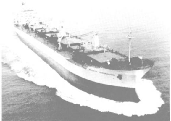
Designed as the largest bulk carrier that can transit the Panama Canal the Maersk Seragoon features a bulb stern and B&W engines.
