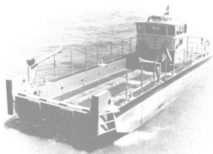
MonArk model 4014 barge built for the C.O.E., Savannah, Ga., is powered by twin 6V53 Detroit Diesels.
