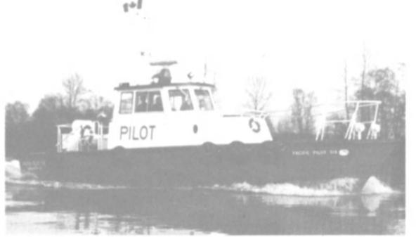
The 49-foot Pacific Pilot Six is powered by Detroit Diesel engines and Maritime Industry "strut drives."
