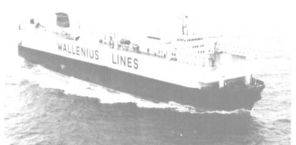
Wallenius car and truck carrier features 13 decks of which 4 are moveable and 3 reinforced trailer decks.
