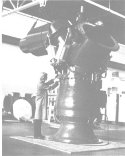
PV/JT1100, 1,000-hp module thruster.
