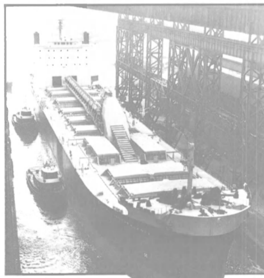
The self-unloading Energy Independence, built by General Dynamics Quincy Shipbuilding Division for New England Collier Co., is the first coal-fired collier built in the U.S. for more than 50 years. All eight conveyor belt doors are by Walz & Krenzer.
