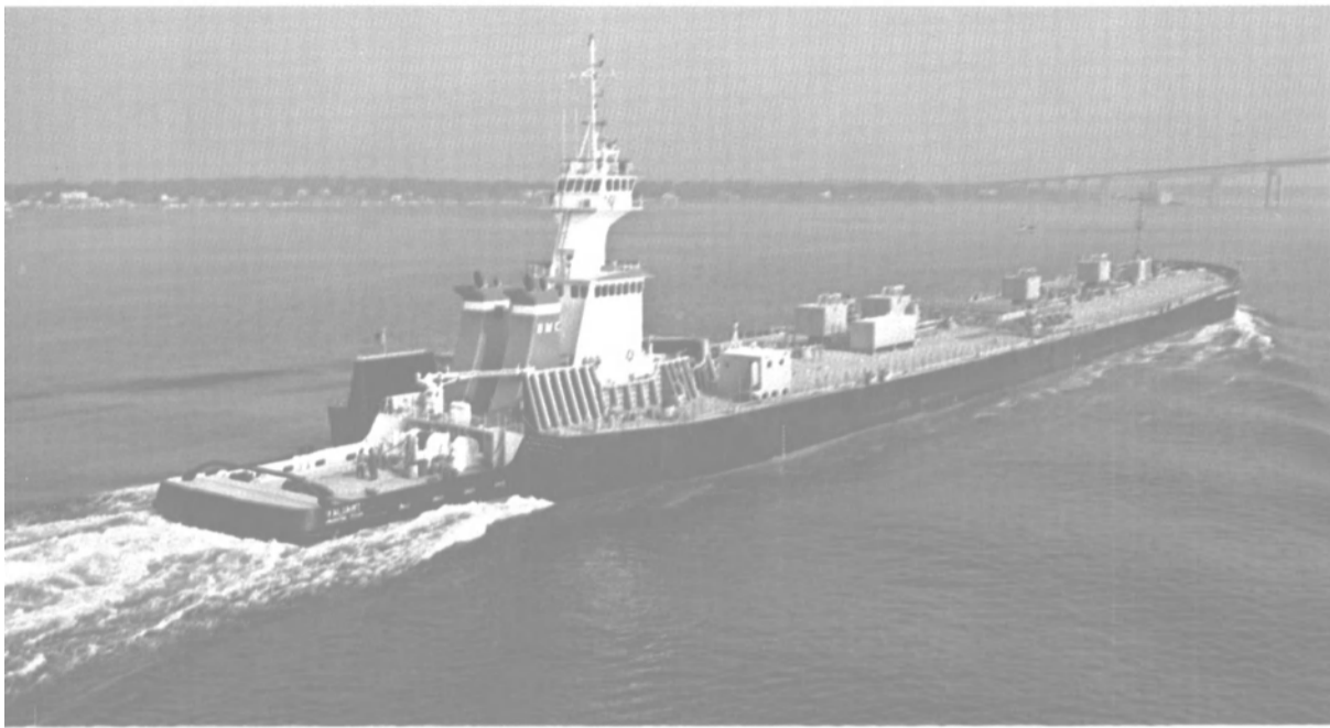
The M/V VALIANT, a deep-notch tug operating with the barge BULKFLEET PENNSYLVANIA, is powered by two Krupp MaK 6MU 551 AK 6-cylinder heavy fuel engines.
