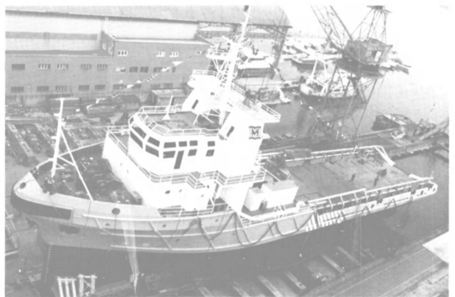
Multi-purpose tug/supply vessel Val Cadore on the ways prior to recent launching at the Viareggio yard of Societa Esercizio Cantieri. Vessel is powered by Wartsila diesels.
