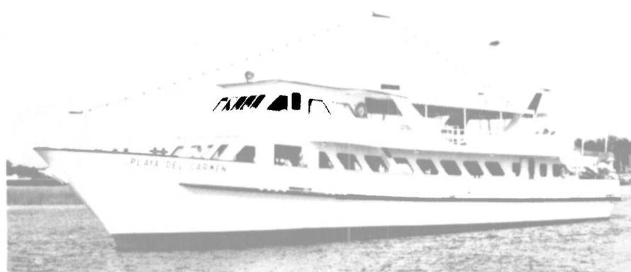
Ferryboat Playa del Carmen carries 600 passengers at 15.7 knots, and is powered by three GM Detroit Diesel 600-bhp engines. Vessel was designed by DeJong & Lebet.
