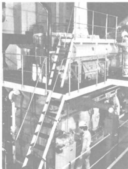
M.A.N.-B&W 3L 58/64 test engine with a cylinder output of 1,215 kw (1,650 hp) at a rated speed of 428 rpm.
