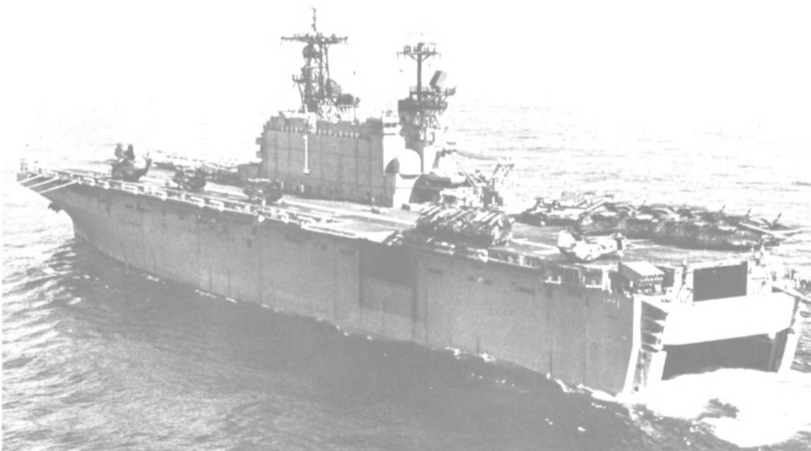
LHD-1 Class will be similar in most respects to five Tarawa (LHA-1) Class general-purpose amphibious assault ships built by Ingalls in the 1970s. The 844-foot LHD-1 will displace approximately 40,500 tons.
