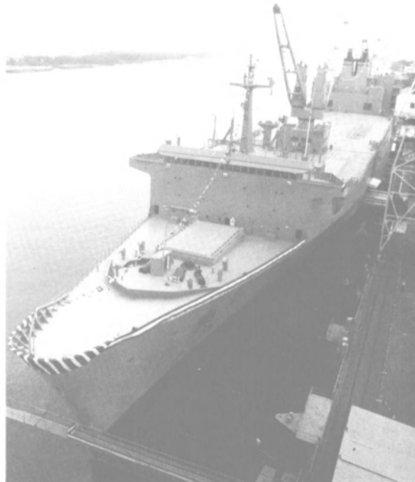
Fast Sealift Ship USNS Antares has been delivered to MSC by Avondale. She is first of three former SL-7 containerships being converted by the New Orleans shipyard.
