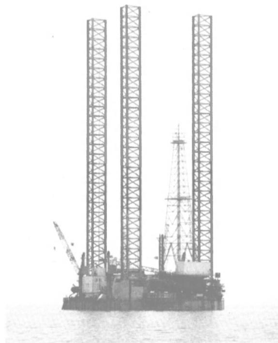
ASRY (Arab Shipbuilding and Repair Yard Company) in Bahrain recently completed, at a cost in excess of \$3 million, an extensive overhaul of the mobile offshore rig Dana, owned by Qatar General Petroleum Company. The rig, a jackup Marathon LeTourneau design built in Singapore, is capable of drilling to 20,000 feet in 250 feet of water.
