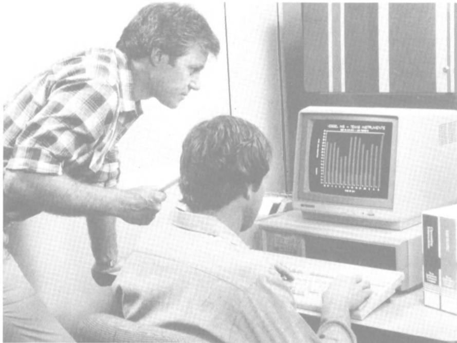
information logged by a TI 8000 Integrated Marine System installed on individual vessels, the system permits managers to download information to a Texas Instruments Professional Computer, and to apply advanced computer spreadsheet capabilities to the analysis of vessel operation.
