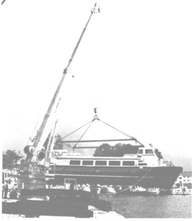
We build one of the original product lines of hydraulically operated, pedestal mounted marine cranes. The line consists of 20 standard models with telescopic and double tapered box booms. Designed for use in a saltwater atmosphere, our cranes provide dependable performance on ships, barges, docks, offshore drilling/production platforms and work boats.
