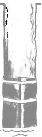
6,000 pounds with a working tension of 1,200 pounds. A dacron jacket and extruded polyurethane layer separate the core from 21 color coded No. 20 FEP insulated conductors. The conductor layer is covered with a foil shield and mylar wrap after which a heavy polyurethane jacket is applied.
