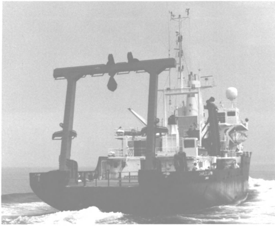
The Mirlees Blackstone-powered Charles Darwin, constructed at Appledore, shows the MacGregor Navire 20-ton gantry.
