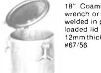
18" Coaming. Available with T socket-wrench or removable handwheel (can be welded in place) for top opening. Spring-loaded lid w/inside handwheel. Coaming 12mm thick — top 11mm. Bosmet drawing #67/56
