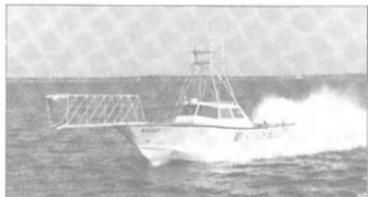
370 HP Caterpillar 3208 turbo-charged diesel. Super-fast. Low wake. Propulsion by an Arneson surface piercing propeller. Speeds to 40 knots. Available in several configurations. Shipable by truck anywhere.
