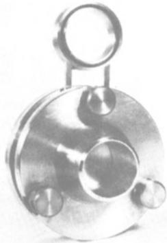
American Piping Products, Inc., manufactures a complete line of quick-acting spectacle blinds, featuring forged-steel bodies. They are designed for marine piping systems which cannot tolerate leakage and are commonly used for cargo segregation, inert gas and ballast piping.
