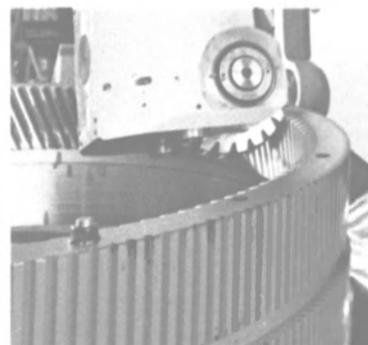
■ Internal hobbing head attachment for internal gears up to 220" pitch diameter.
