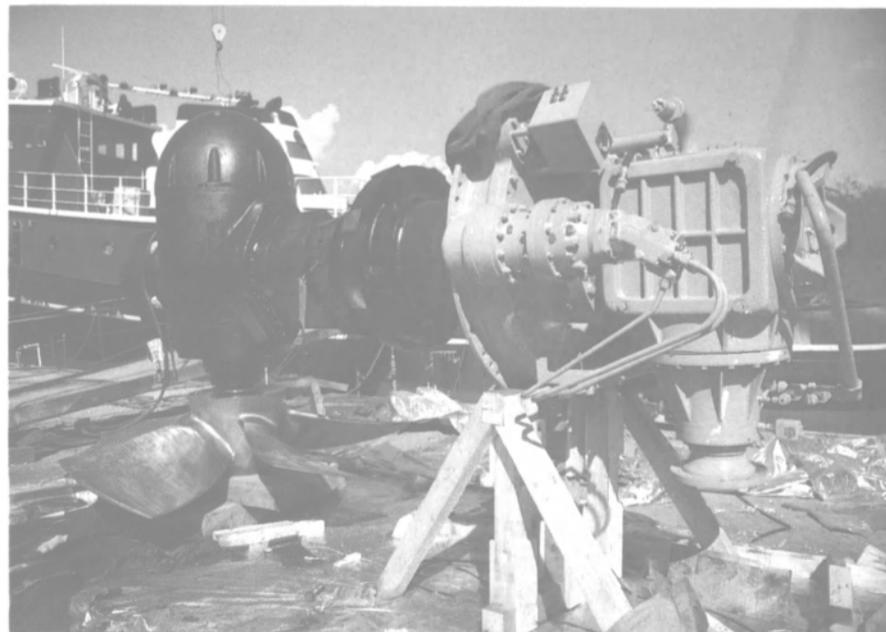
control of thrust and direction. The propellers are enclosed in nozzles to further enhance the bollard pull of the vessel.
