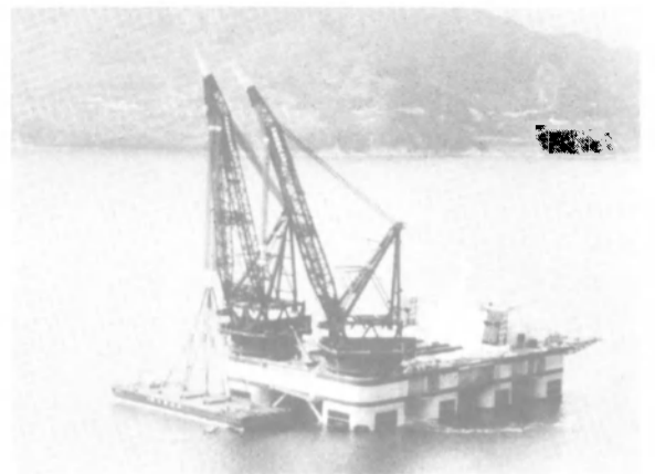
Two American cranes aboard McDermott's semisubmersible crane vessel DB 102 set world record for heaviest marine lift during sea trials, picking up a barge weighted at 7,260 short tons. The vessel is equipped with two Amhoist cranes capable of 12,000-ton lift when operated in tandem.
