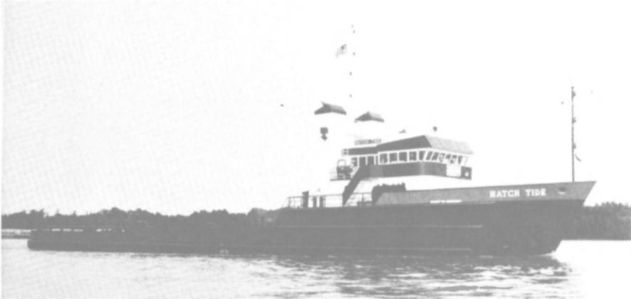
The Hatch Tide's maneuverability was increased by the addition of a 550-hp Schottel bow thruster.
