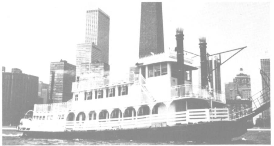
Sternwheeler Betsy Ann, converted to an excursion vessel in 1982, is powered by two Hagglund hydraulic motors driven by hydraulic pumps/diesel engines.
